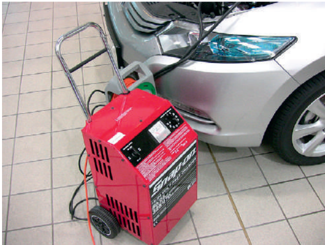
Figure 2.344 Hybrid cars still use a normal 12V battery
